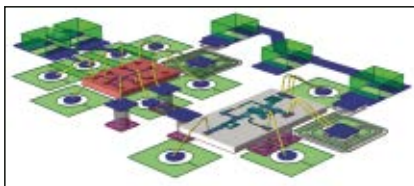
▲ Fig. 12 SiGe PA combined with a PHEMT via a coupler.
